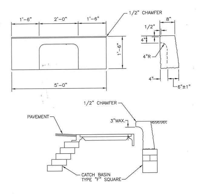
NOTES: 1. SHALL BE IN ACCORDANCE WITH SECTION 906 OF THE R.I. STANDARD SPECIFICATIONS. 2. TOP SURFACE TO BE DRESSED BY SAW. REMAINDER MAY BE QUARRY SPLIT.
