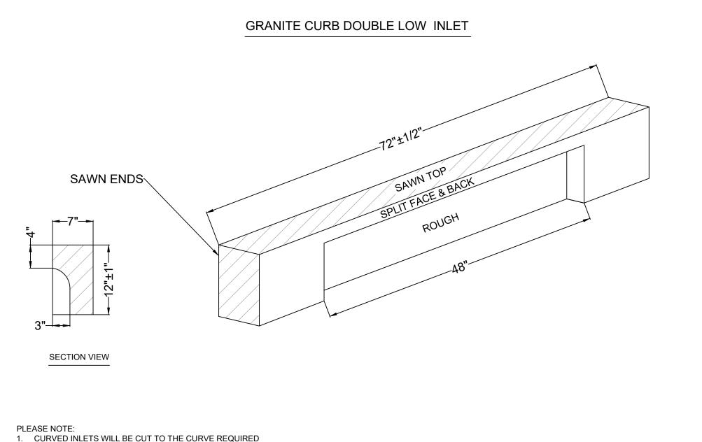
2. JOINTS WILL BE CUT ON RADIAL LINES
